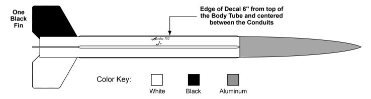
Remove the nose cone and set aside. Mask off the entire model except for one fin to be painted black. The remainder of the body and two of the fins should be totally covered. Paint the exposed fin black and let dry.
