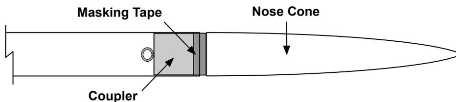
Mask off the black fin to prevent any overspray and paint the nose cone aluminum (or silver). When dry remove all the masking as well as the tape from the coupler.
