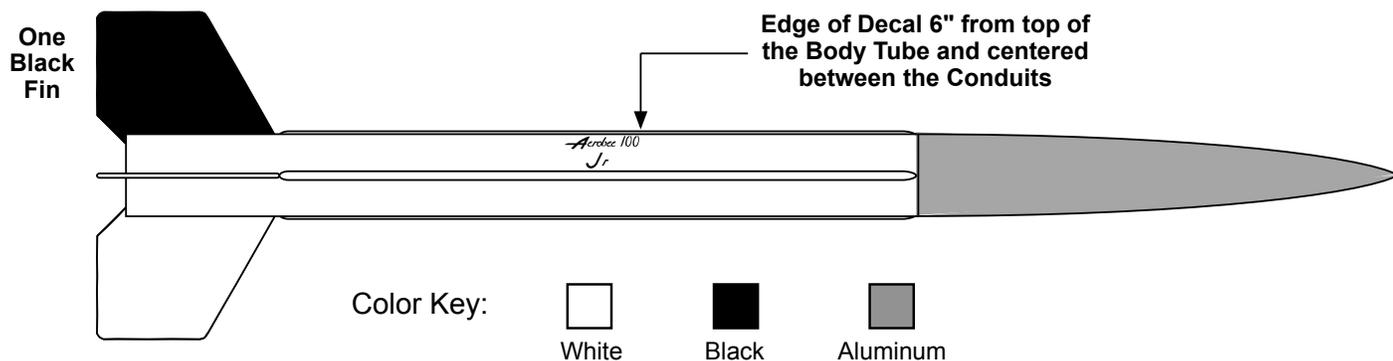
Remove the nose cone and set aside. Mask off the entire model except for one fin to be painted black. The remainder of the body and two of the fins should be totally covered. Paint the exposed fin black and let dry.
