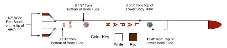
Mask off the entire body of the model that is to remain white and each fin except for the tips of each fin that will be painted red. Also keep the nose cone exposed (note: if you did not glue the cone into place you can simply remove it and paint it separately).
