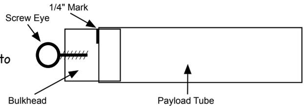
3) Thread the screw eye into the center of the bottom of the bulkhead. Remove the screw eye and put some glue (wood glue is fine for this) into the hole. Thread the screw eye back into the hole and allow to dry.
