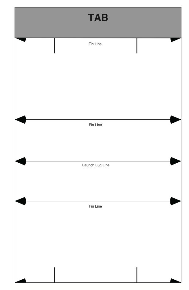
T-2.6 Three Fin Tube Marking Guide
